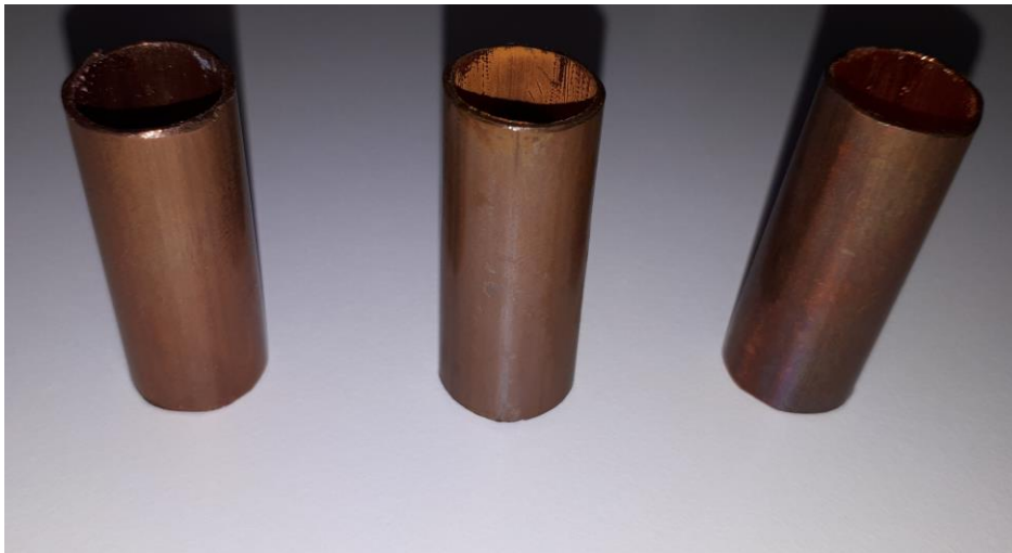
Left: untreated coil / middle: stored in 0,5% v/v Virocid / right: control stored in tap water
