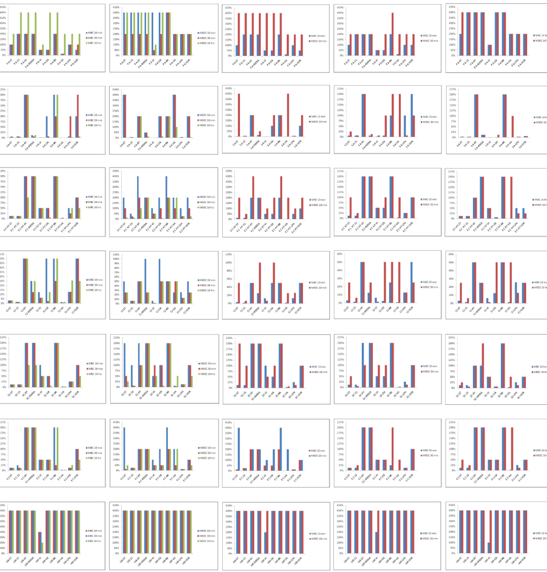
Figure 3. These graphs show the MBEC and MBC values for the tested biocides (Table 2) against the tested strains (Table 1) at three different time exposure; 10 minutes, 30 minutes and 16 hours. VI, Virkon®, LPH, Environ LpH®, IS, 1-Stroke®, OX, Oxonia Active®, ST, SterBac KQ-12®, 400SA, 400 Sanitizer®, XY, XY-12® and BK, BevoKlene®, VOR, Vortexx® and VA, Vantocil®
